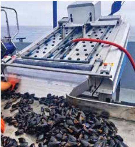
Harvested mussels run through a grader machine that sorts them by size and debeards them.
