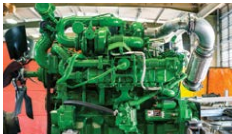
A PowerTech™ PVX 6.8L Interim Tier 4/Stage III B engine is assembled for installation into a dual-fan Super 80 sprayer.
